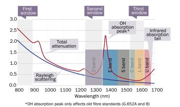
Figure 1: Silica-based fibre attenuation profile as a function of wavelength [Source: Analysys Mason, 2022]
