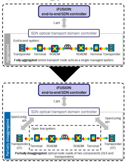
Figure 3.1: Telefónica's partial optical network disaggregation architecture
