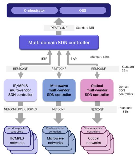
Figure 2.1: Telefónica 's SDN reference architecture for transport
