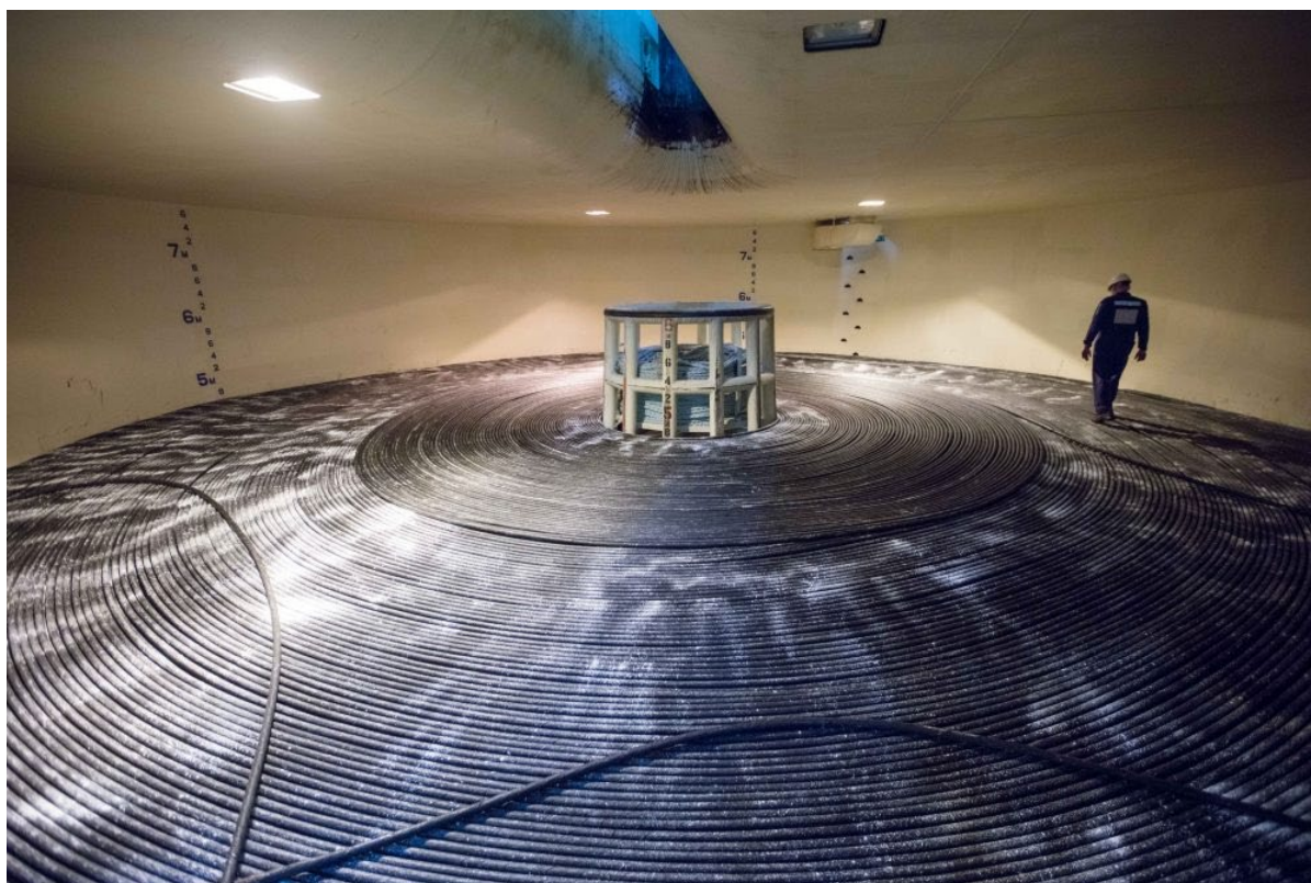
Figure 5.9: The Marea cable coiled on ship [Source: Photo by RUN Studios, provided by Microsoft, 64 2017]
