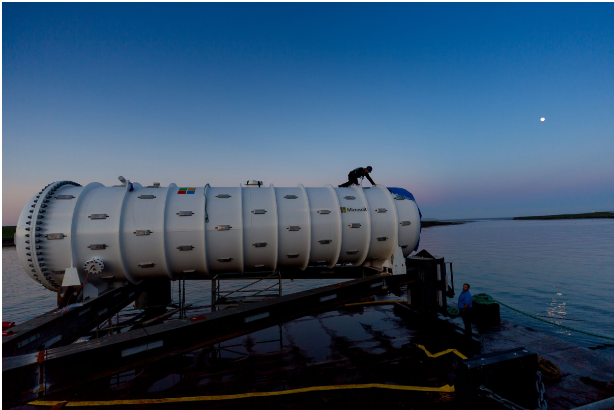
Figure 6.3: Microsoft Project Natick's Northern Isles data-centre being prepared for deployment [Source: Photo by Scott Eklund/Red Box Pictures, provided by Microsoft, 107 2018]
