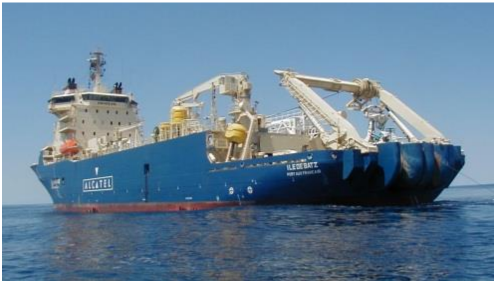
Figure 4.7: The Ile de Batz, a submarine cable laying ship [Source: WIOCC, 2014]
