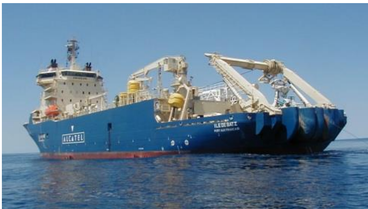
Figure 1.4: The Ile de Batz, a submarine cable laying ship [Source: WIOCC, 2014]
