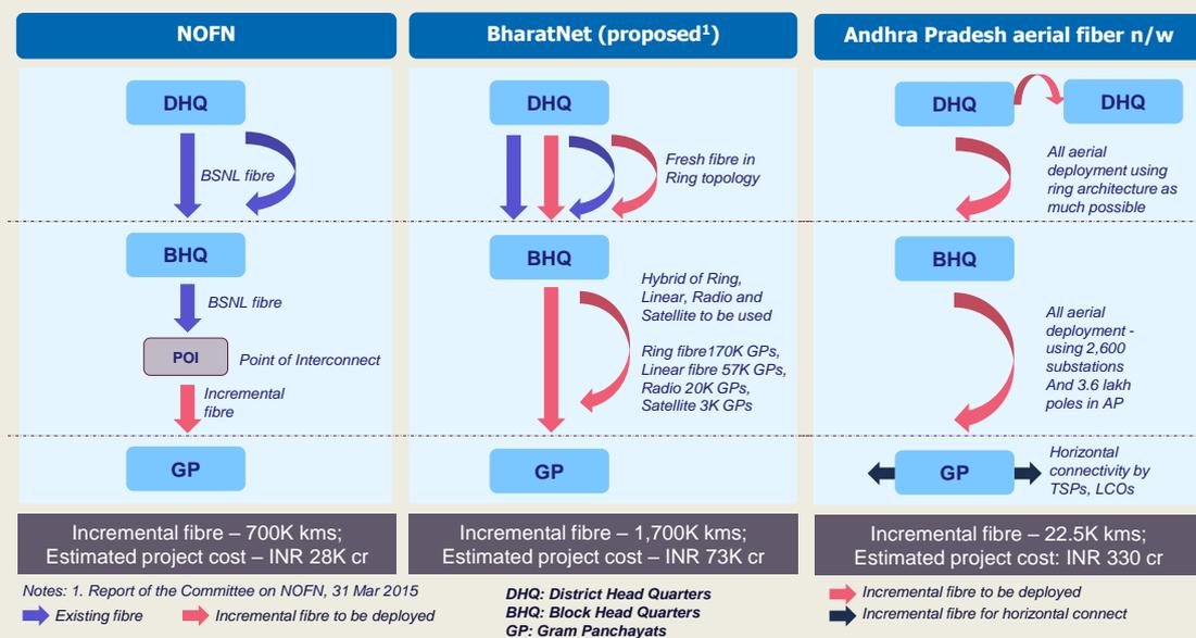
This model has reduced the cost for deployment significantly (from an estimated USD600 million to USD50 million)\* thanks to the use of aerial fibre (rather than underground deployments) and the reuse of existing fibre and civil infrastructure.
